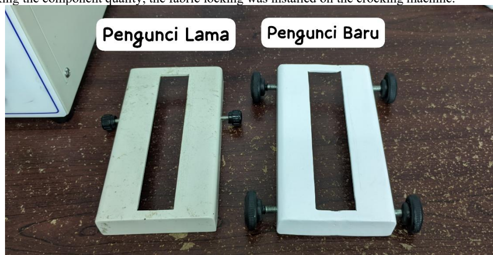
Figure 5: Comparison of the old and new locking system.
