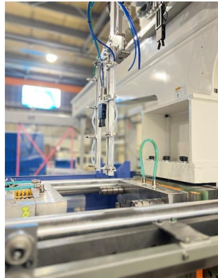
Fig. 7 EOAT insalled on robot injection machine
