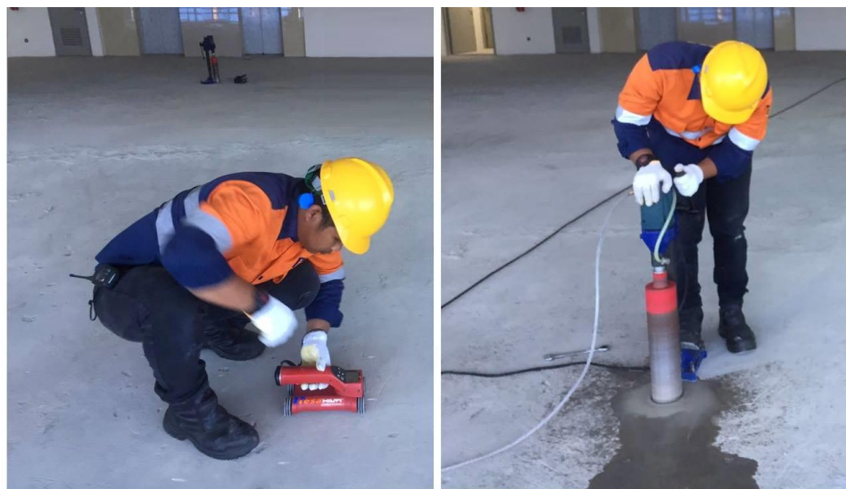
Fig. 2 Rebar scanning (left) and concrete core sample collection (right)
