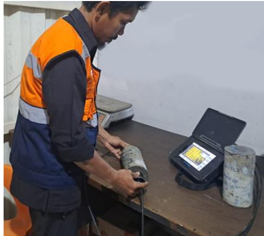
Fig. 3 Ultrasonic pulse velocity data collection on concrete core sample
